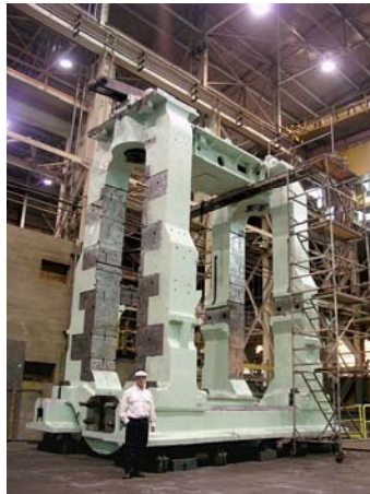
160" plate mill retrofit – Housing, chocks & Quick roll change system
