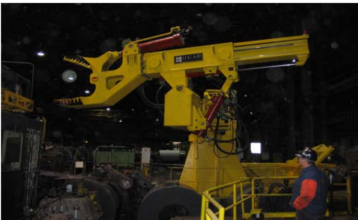
Custom designed pup coil removal system to increase productivity and safety
