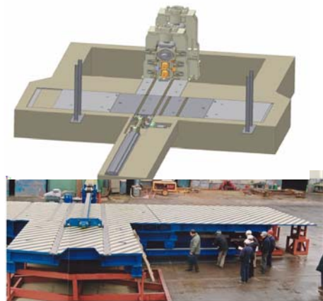
160" plate mill retrofit – Housing, chocks & Quick roll change system
